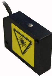
The Laser ride height sensor gives a 0.2 to 4.8V output which is proportional to its displacement above the ground. The displacement is calculated by triangulation from the position of the reflected beam.
